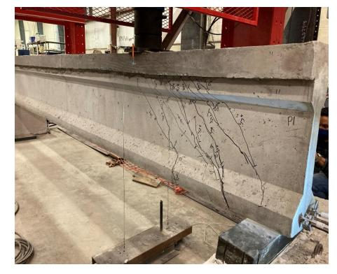
Prestressed beam with bond-shear cracks
