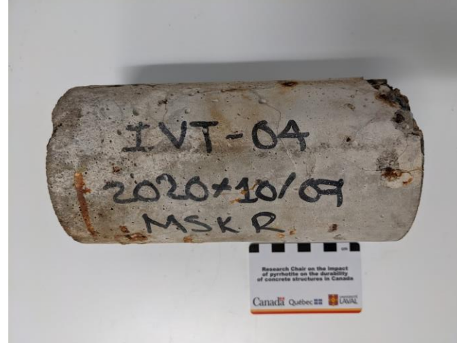
Chloride Impregnation (14d) + Impressed Voltage (7d)
