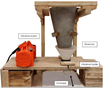
Prototype of vibration based concrete 3D printer
