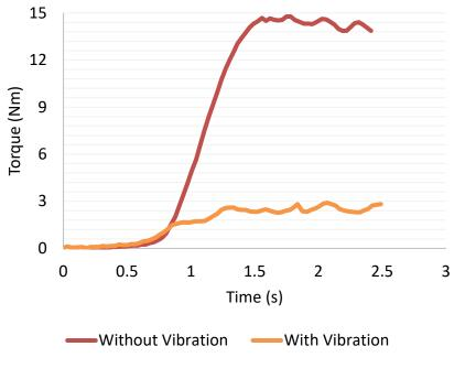
Torque versus time: sample raw data - ICAR stress growth test
