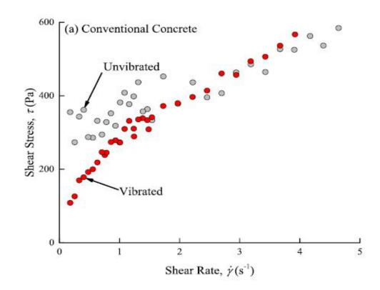
Shear stress vs. Shear rate of conventional concrete with and without vibration. (Koch, Castaneda, Ewoldt, & Lange, Cem. Concr. Res., vol. 115, pp. 31-42, Jan. 2019)
