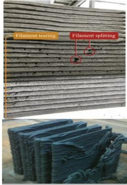
Defects in 3D Printed concrete (Buswell, Leal de Silva, Jones, & Dirrenberger, Cem. Concr. Res., vol. 112, pp. 37–49, Oct. 2018)
