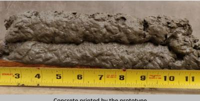
Concrete printed by the prototype
