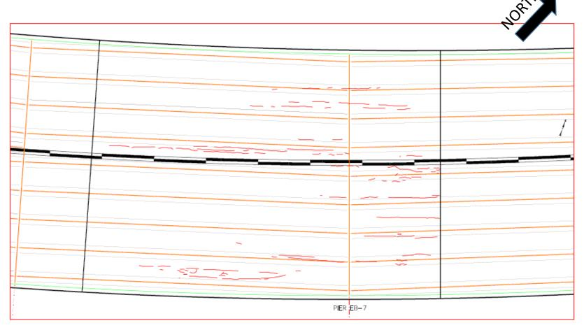
PLACEMENT 6 - SPAN 7, 8 CRACK MAPPING
