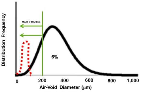
A 1%-dose (by volume) of 40-µm spheres produces 22,000,000 spheres per cubic foot of concrete
