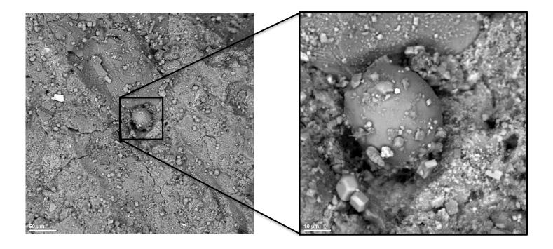
• Fracture surface of concrete (1% MS) saturated, frozen and viewed on cryostage in SEM
