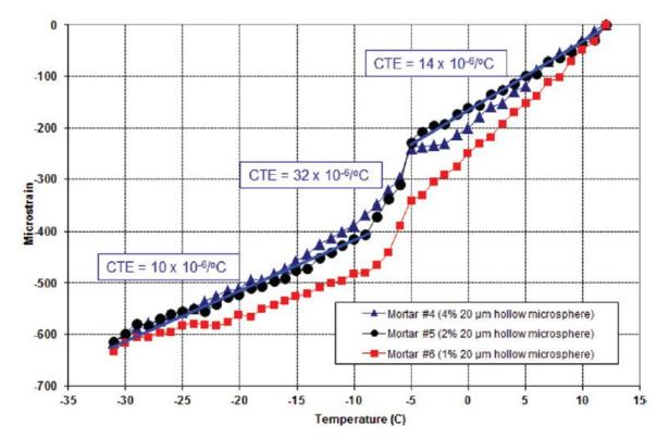
Microstrain as function of temperature during freezing for mortar containing 1, 2, or 4% by volume of 20  $\mu$ m diameter hollow (compressible) microsphere during first cycle of testing.
