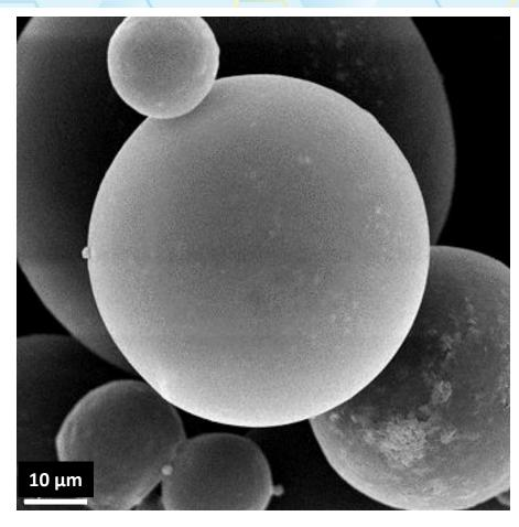
Polymeric microspheres with nominal diameter of 40  $\mu$ m Note: 1  $\mu$ m = 40 x 10<sup>-6</sup> in.
