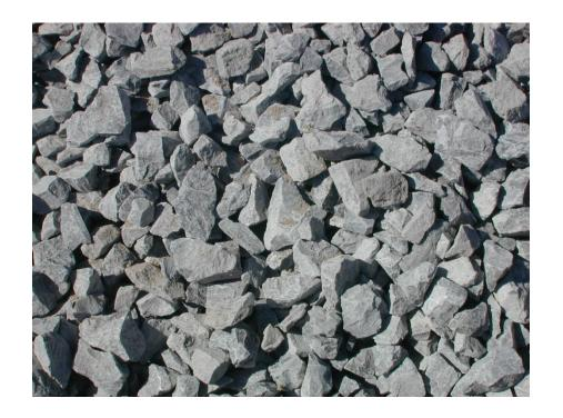
For most common applications, no more than 10% should pass a 3/4" sieve and no more than 2% should pass a 1/2" sieve
