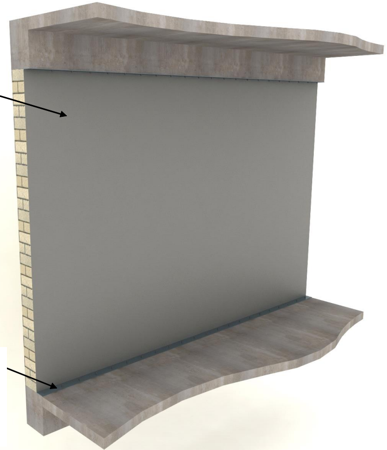
FRP panel with concrete anchor bolts (top and bottom)
