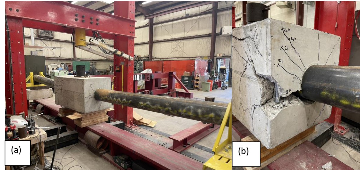
Specimen 6 (a) loading set up and (b) pullout failure
