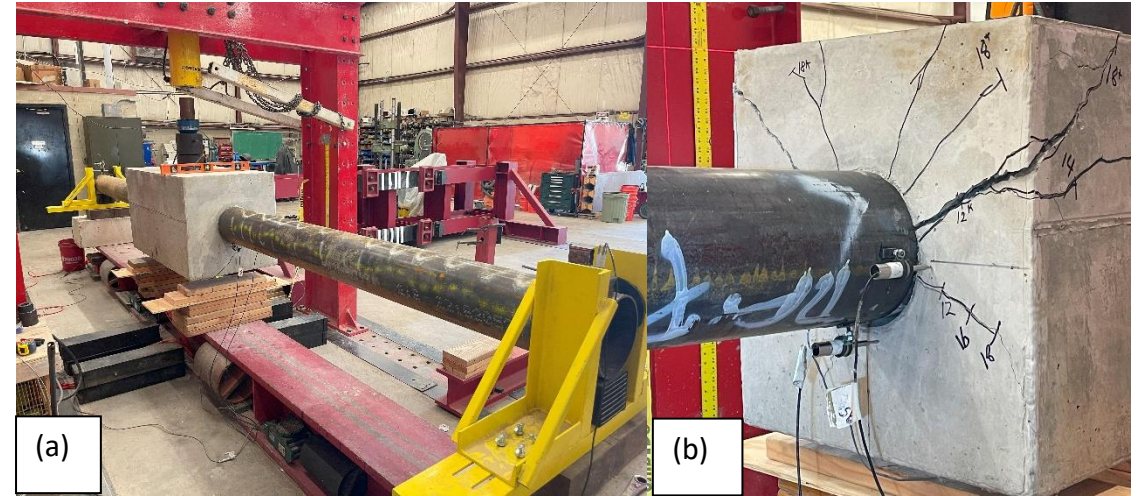
Specimen 5 (a) loading set up and (b) pullout failure
