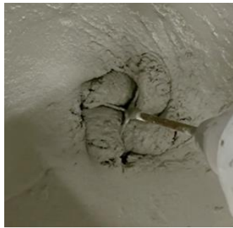
(a) Hand vane shear test
