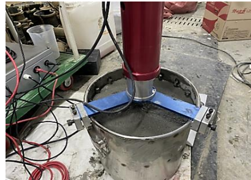
(b) Rotational rheometer test
