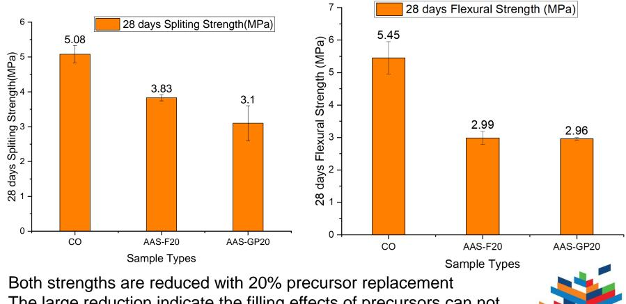
The large reduction indicate the filling effects of precursors can not contribute to the tensile and flexural strength.
