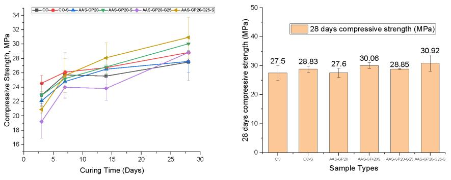
The compressive strength improves with reinforcement of recycled tire steel fibers
