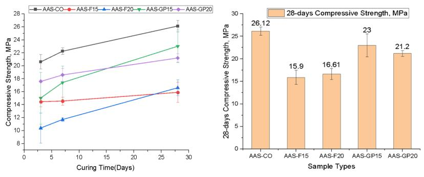
Samples with 15% glass powder has the comparable compressive strength as control
