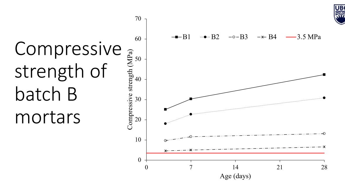
Minimum required strength of non-load-bearing masonry unit is 3.5 Mpa (ASTM C129)
