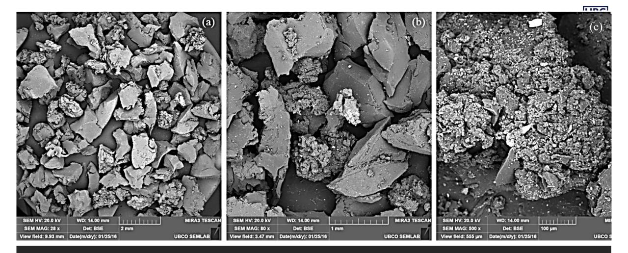
Crumb rubber particles at magnification levels of (a) 28x, (b) 80x, and (c) 500x using Scanning Electron Microscope (SEM)
