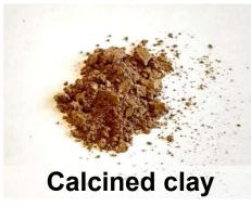
Burned at much lower temperature than clinker and small process emissions
