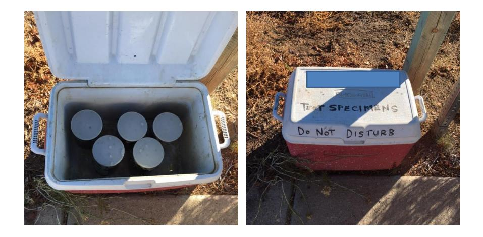
Improper curing per ASTM C-31 You could loose 1000 psi in 28 days
