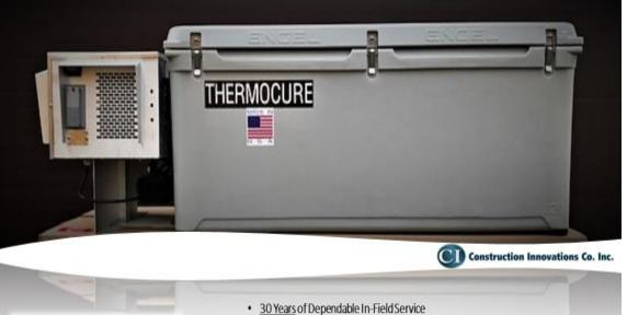
Thermocure II Concrete Cylinder Curing Box
