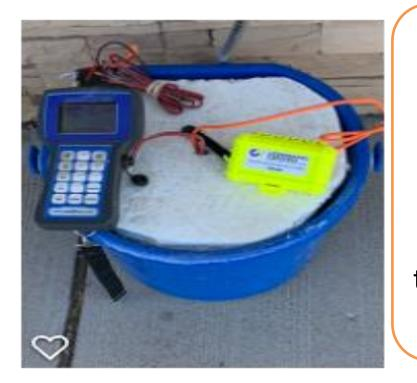
Command center and intellirock sensors use to record temperatures
