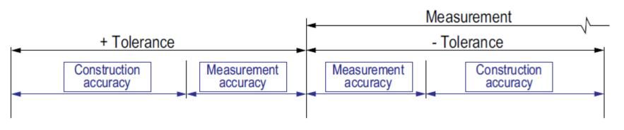
A specified tolerance includes a measurement accuracy and a construction accuracy
