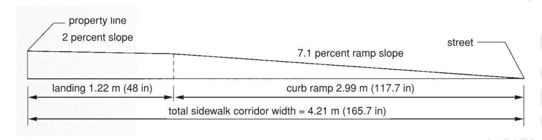
"Therefore, rather than using 8.3 percent for designing curb grade, a grade of 7.1 percent is recommended to allow a construction tolerance."
