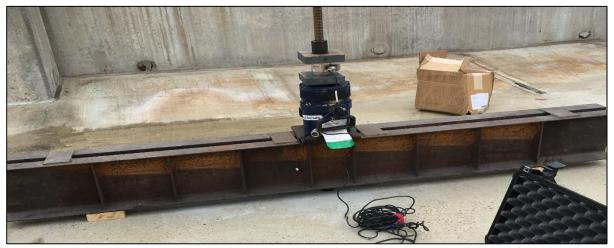
Steel Spreader Beam with High Strength Williams Bar
