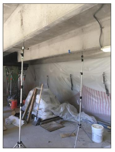
Dial Gages at Underside of DT Beams
