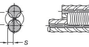
Indirect Butt Splice Weld:
