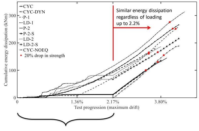
Variation in energy dissipation due to the different loading protocols carried through until failure.
