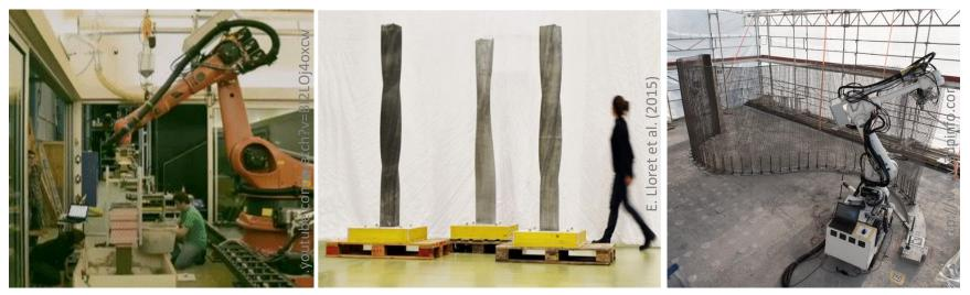
Smart dynamic casting and mesh mold (ETH Zurich)
