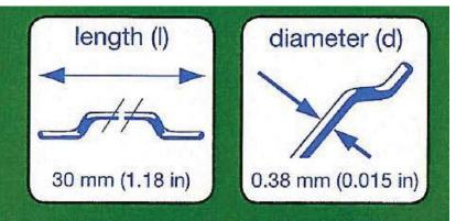
DIAMETER: 0.015" LENGTH: 1.18" STRENGTH: 445 KSI MATERIAL: ASTM A820 DOSAGE: 1.5% BY VOLUME  $= 200 \#/YD^3$
