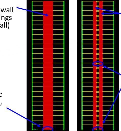
Concrete shear wall with openings (Coupled Wall)
