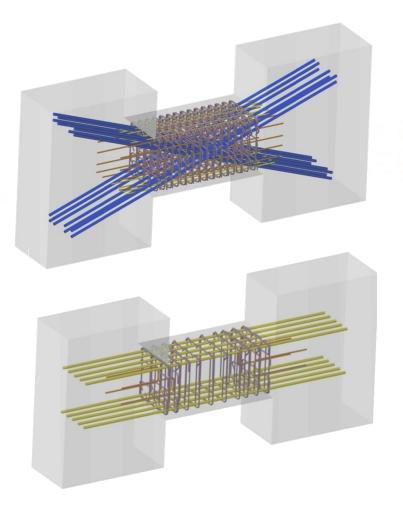
Diagonally Reinforced Concrete Coupling Beam
