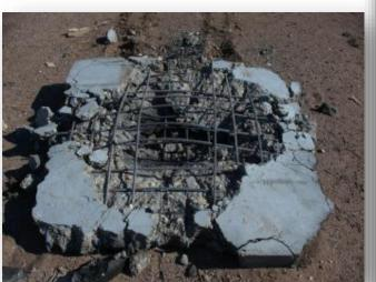
Rebar Only 2 Layers #3 at 100 mm 100 mm thick Panel
