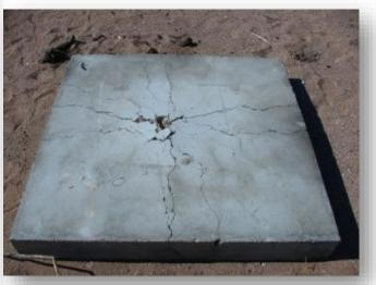
TSMR 5-25 at 30 kg/m<sup>3</sup> 2 layers #3 at 150 mm 100 mm thick panel
