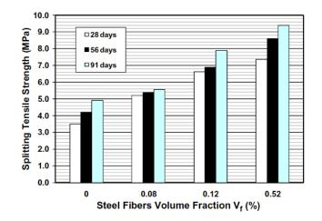
Fig. 5. Splitting tensile strength for different steel fiber volume fraction.
