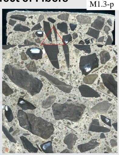
•M0.0p: No restraint; cracks opened, extended to paste matrix and gel flowed to paste
