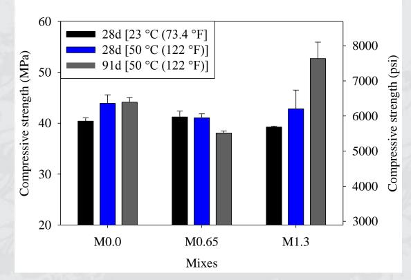
•fc' increased with accelerated conditioning. fc' increased significantly for M1.3 mix (by 34% of the 28d strength).
