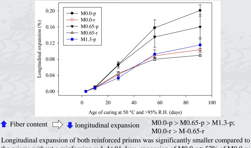
the prisms without a reinforcing rod. At 91 days, expansion of M0.0-r  $\approx$  52% of M0.0-p; expansion of M0.65-r  $\approx$  55% of M0.65-p
