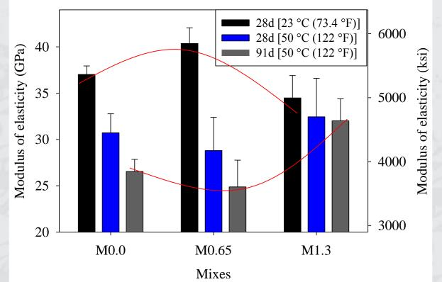
•Ec decreased with accelerated curing. Max. degradation was 29% for M0.0 and 38% for M0.65.
