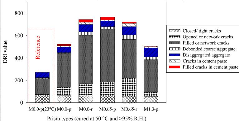
•DRI values for the specimens cured at 50 °C (122 °F) were significantly greater compared to the reference specimen.
