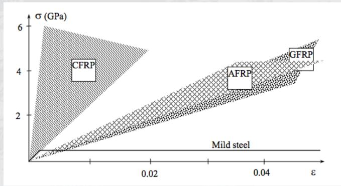
CFRP = Carbon FRP AFRP = Aramid FRP GFRP = Glass FRP
