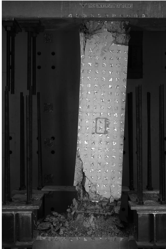
Gr 60 Pushed after lowering axial load.
