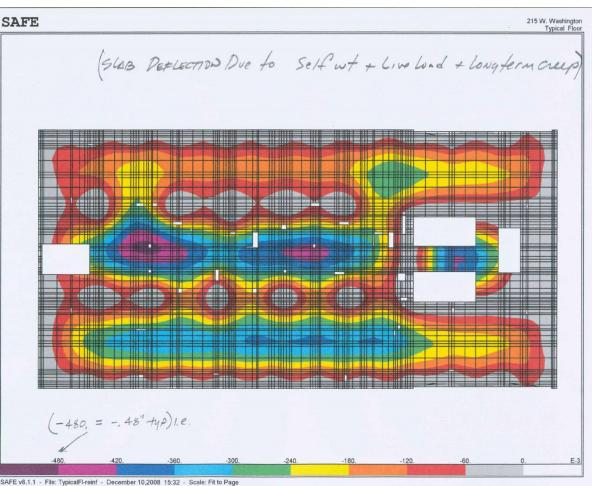
Cracked Deformed Shape (SERVICE) - Kip-in Units
