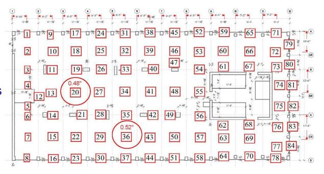
Average Measured Slab Deflection of Points 20 & 36 of Level 15 thru 50 at 3.5 to 4 weeks of age.
