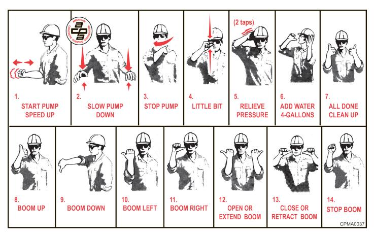
Fig. 1.1—Concrete pump operation hand signals. (Figure courtesy of American Concrete Pumping Association.)
