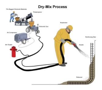
*Fig. 1.1.1—Dry-mix shotcrete process.*
