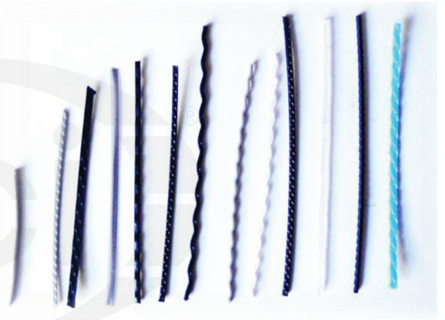
Fig. 3.2b—Examples of synthetic macrofibers.
