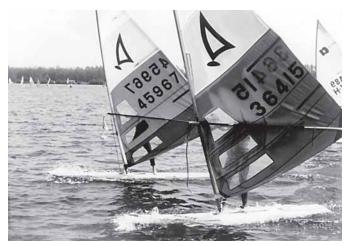
The first concrete windsurfer race was held at Den Bosch, The Netherlands, in 1985. One board was built from ferrocement and one from glass-reinforced concrete (GRC). *ACI archives. Photo courtesy of International Ferrocement Information Center, Bangkok.*
