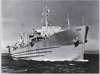
Dry-cargo, self-propelled concrete ship built during World War II by U.S. Maritime Commission. The hull shell was 6-1/2 in. (165 mm) and contained from three to five layers of closely-spaced reinforcing. Cover over the steel was 3/4 in. (19 mm) on the outboard face and 1/2 in. (12 mm) on the inboard face.
