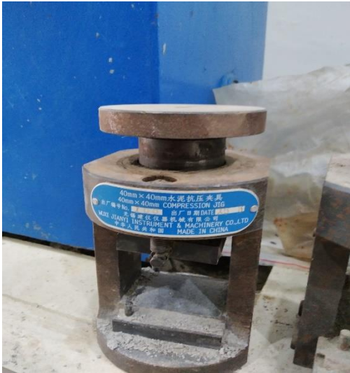
(a) Compression Device for Mortar
