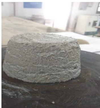
(c)Mortar after lifting the mold
