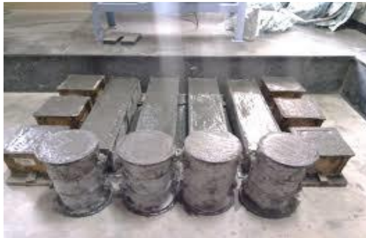
FIG-19 CASTING OF SPECIMEN
