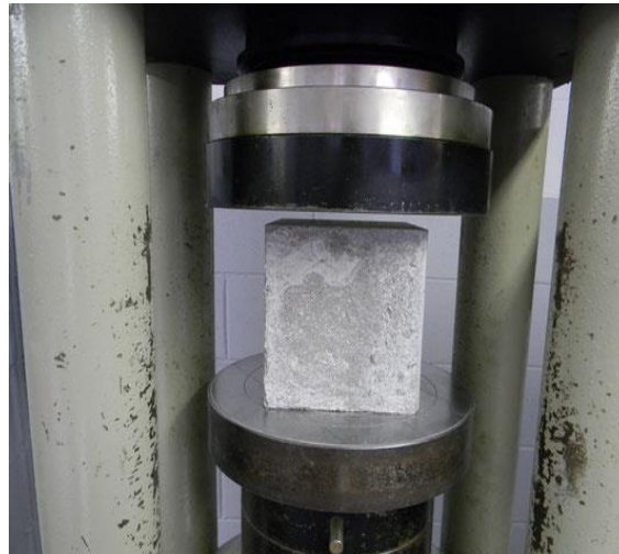
FIG – 8 COMPRESSIVE TEST ON CUBE
