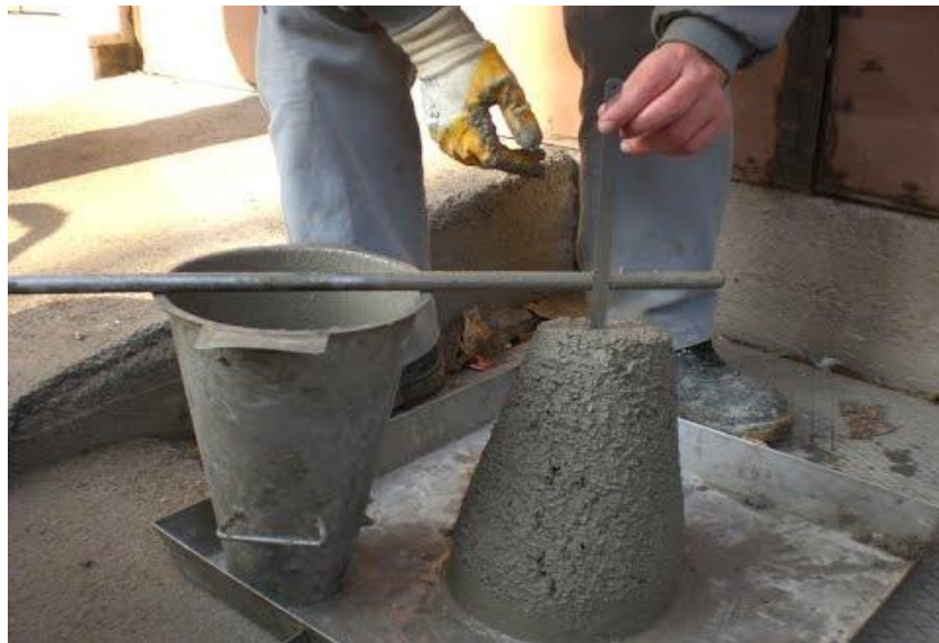
FIG- 18 SLUMP CONE TEST
