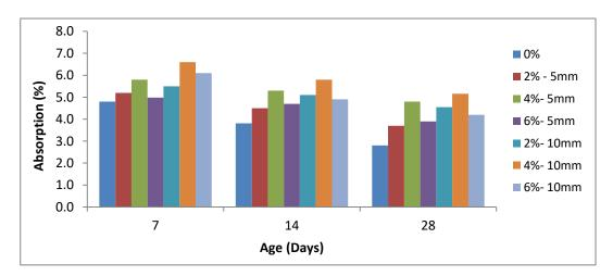
Fig. (17)The effect of rock wool on absorption of ferrocement mortar using CO<sub>2</sub> curing.
