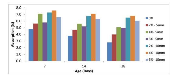
Fig. (16)The effect of rock wool on absorption of ferrocement mortar using water curing.
