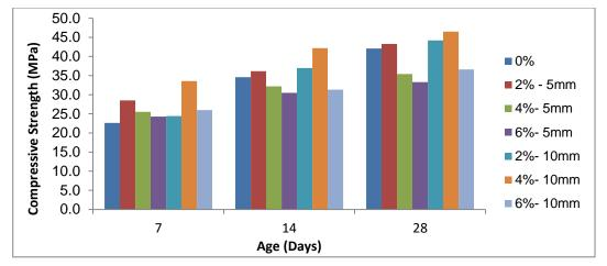
Fig. (9) The effect of rock wool on compressive strength of ferrocement mortar with CO<sub>2</sub> curing.
