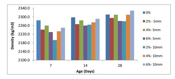
Fig. (6) The effect of rock wool on density of ferrocement mortar with water curing.
