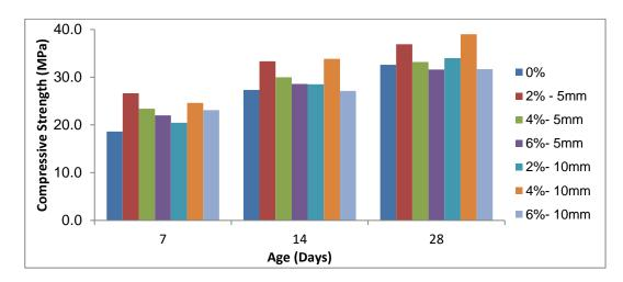
Fig. (8) The effect of rock wool on compressive strength of ferrocement mortar with water curing.
