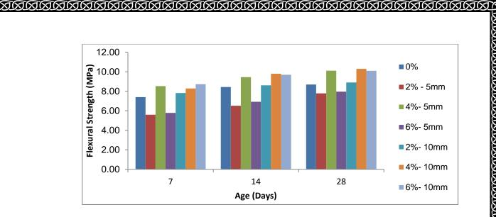
Fig. (10) The effect of rock wool on flexural strength of ferrocement mortar using water curing.
