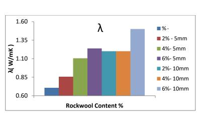
Fig. (14) The effect of rock wool on thermal conductivity of ferrocement mortar using  $CO_2$  curing.
