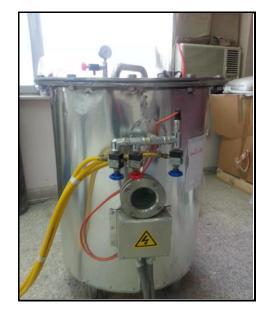
Fig. (2) Carbonation chamber machine
