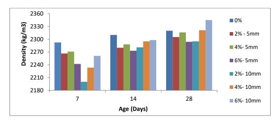
Fig. (7) The effect of rock wool on density of ferrocement mortar with  $CO_2$  curing.
