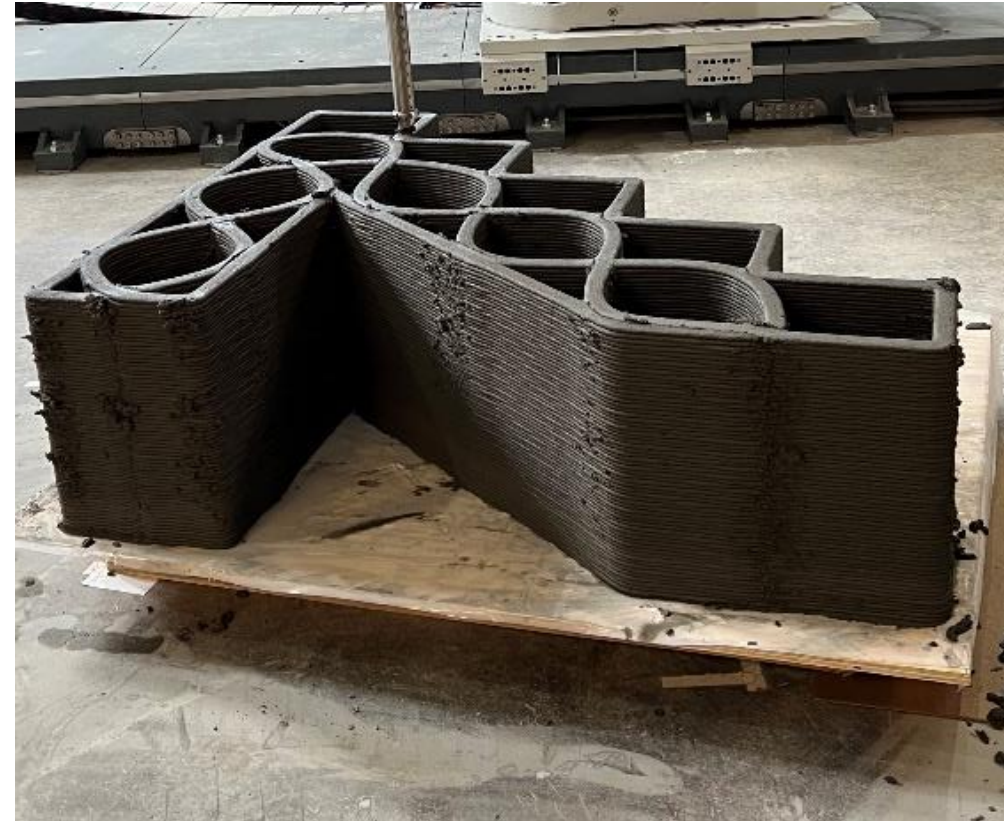
Stacked Layers 32 inches printed in one continuous session
