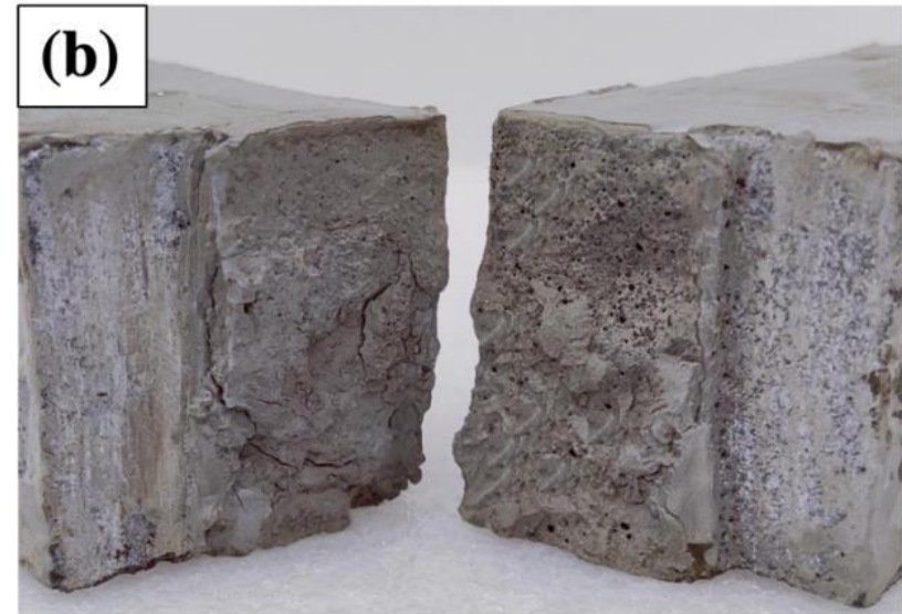
GNP Reinforced Biochar-OPC Mortar
