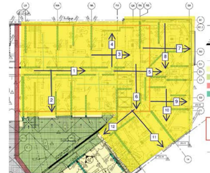
Fig. 1: The yellow shaded area indicates the portion of the podium level slab where 12 sample measurements lines were marked for use in F-number analysis. The lines varied in length from 20 to 35 ft (6 to 11 m). Point coordinates of the start and end of each line were measured using a total station, and these coordinates were provided to each participant. Eight participants performed a laser scan on the lines on two separate days and provided composite F-numbers determined per ASTM E1155 in addition to information on each sample measurement line. For comparison, a Type II device (Dipstick®) was used to collect data twice on the same sample measurement lines
