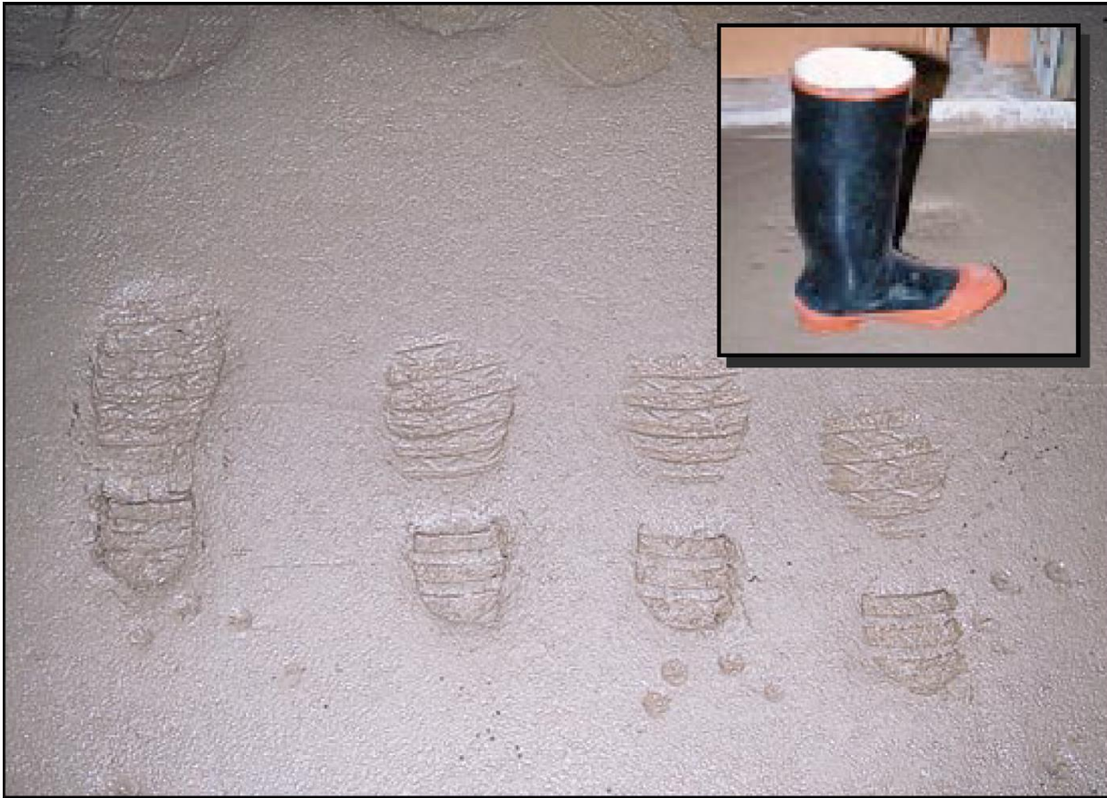
Figure 1. Concrete is generally considered to be ready for floating when finishers leave a ¼-inch-deep footprint in the surface. Using a boot filled with steel shot (inset) to produce footprints, we found that 2½-inch-slump concrete placed on a stone base was ready for floating about 45 minutes earlier than the same concrete placed directly on a vapor retarder.
