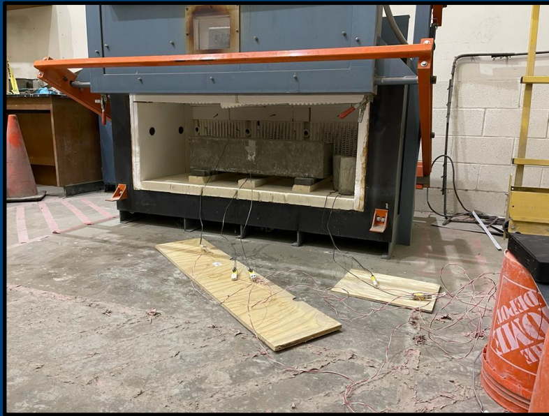
Fire Exposure of specimens: ASTM E119
