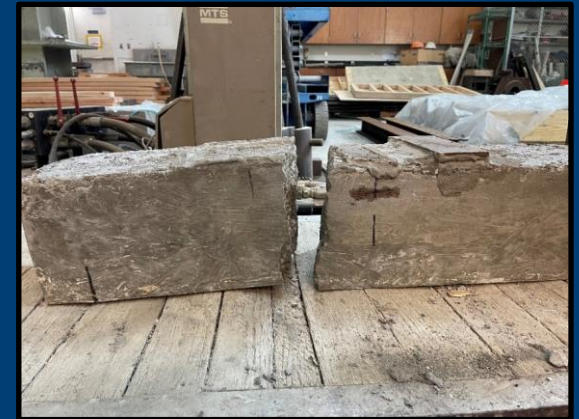
Fracture pattern at room temperature
