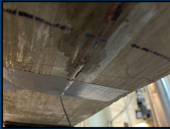
Failure modes at elevated temperature
