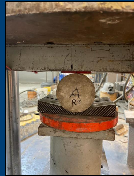
Split Tensile Strength Test: ASTM C496
