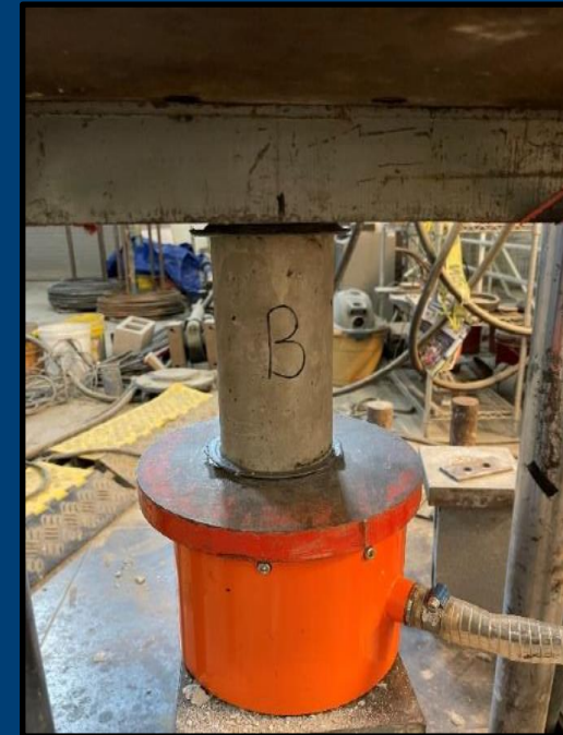
Compressive Strength Test: ASTM C39
