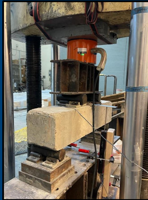
Three-point bending Flexural Test: ASTM C78
