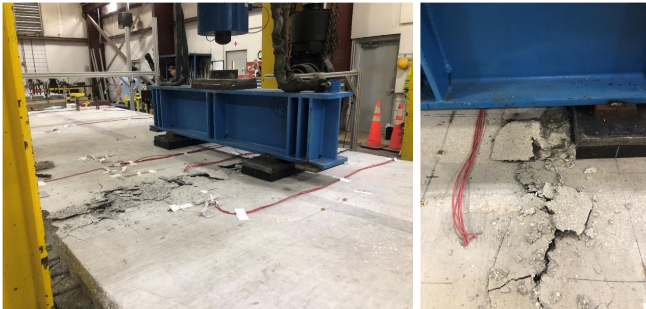
Compression block crushing across joint in FIU-1/2 (Same occurred in FIU-4/5)
