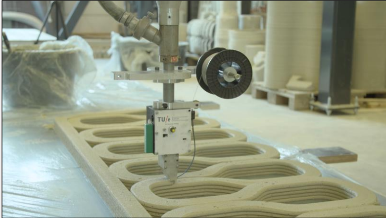
17 Reinforcement of Layer-Extrusion 3D Concrete Printing
