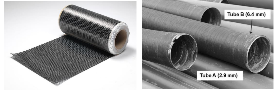
Fig.1. CFRP wrap 1 and filament wound FRP tubes 2 .
