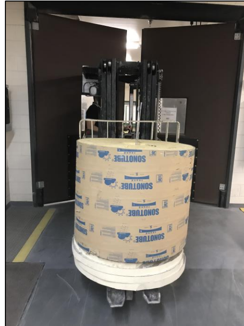
Moved to calorimeter chamber within 30 minutes from start of mixing time
