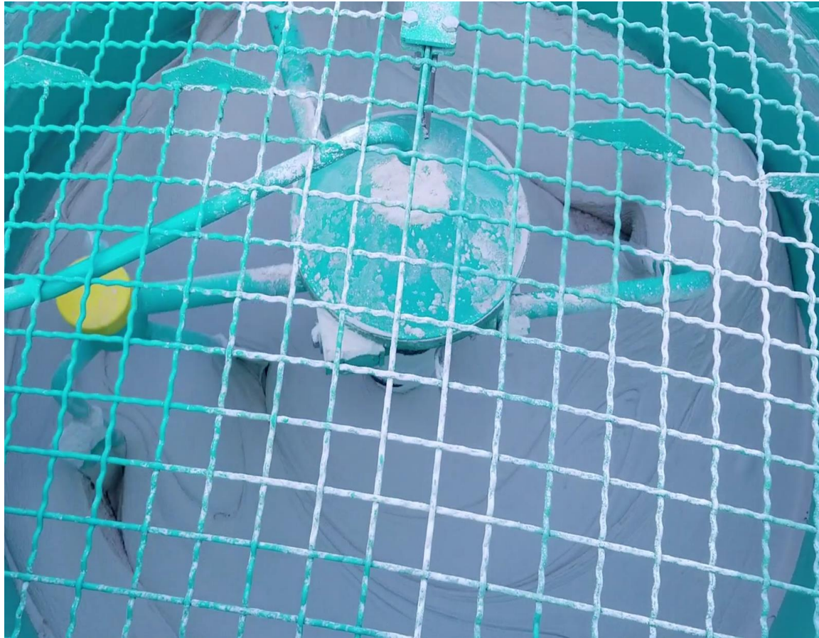
UHPC Mix at UH Structural Lab
