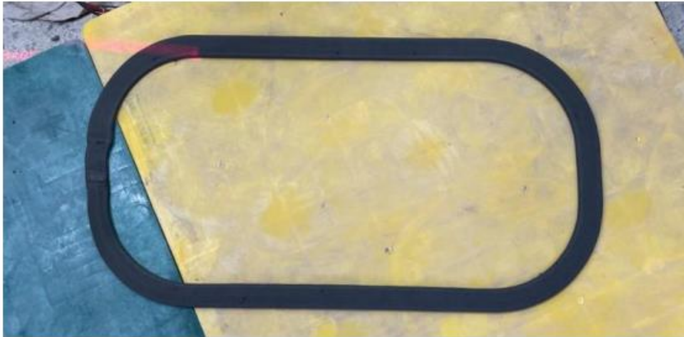
Figure 5-13 Shape of extruded concrete filament after printing
