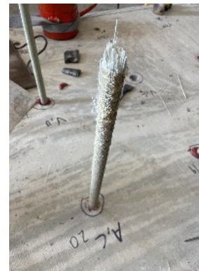
GFRP anchor rupture
