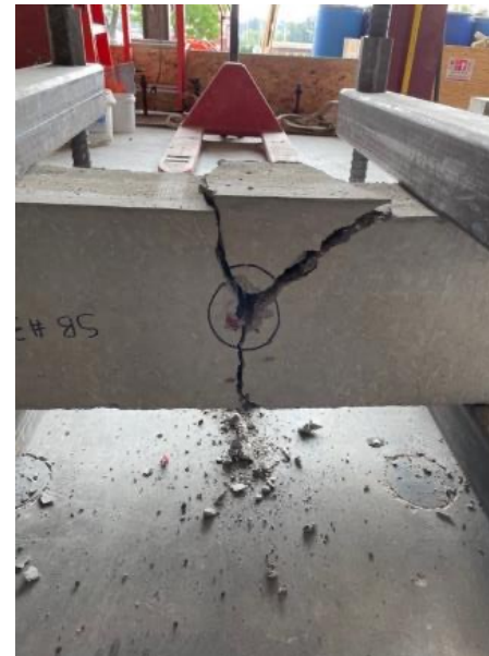
Typical shear failure in concrete with steel bar
