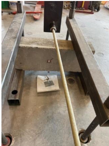
Typical shear failure in GFRP bar
