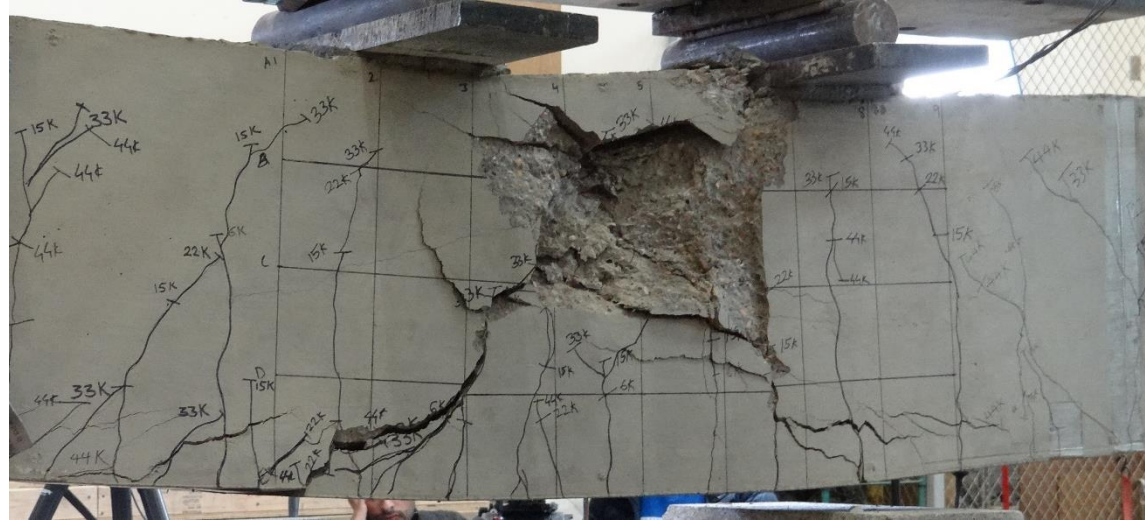
RC #2 beam (Plain Concrete + BFRP bar)
