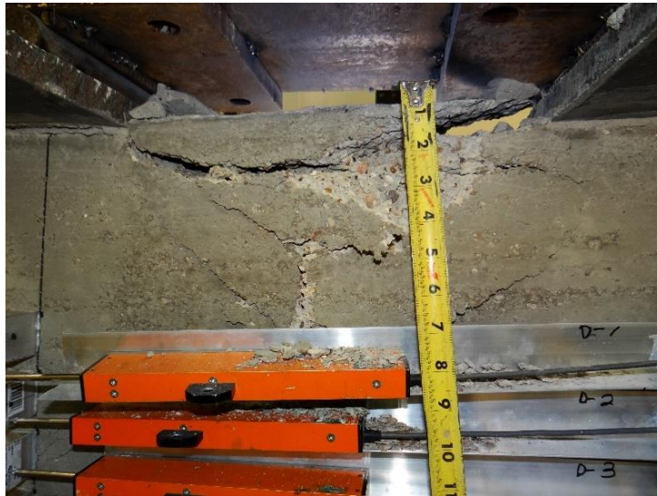
RC #1 beam (Grade 60 steel)
