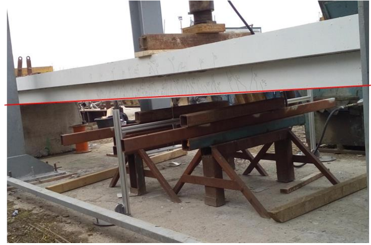
Almost perfect elastic recovery at the end of the test
