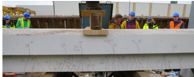
Contribution of polypropylene fibres in distributing the cracks: short spacing and small opening
