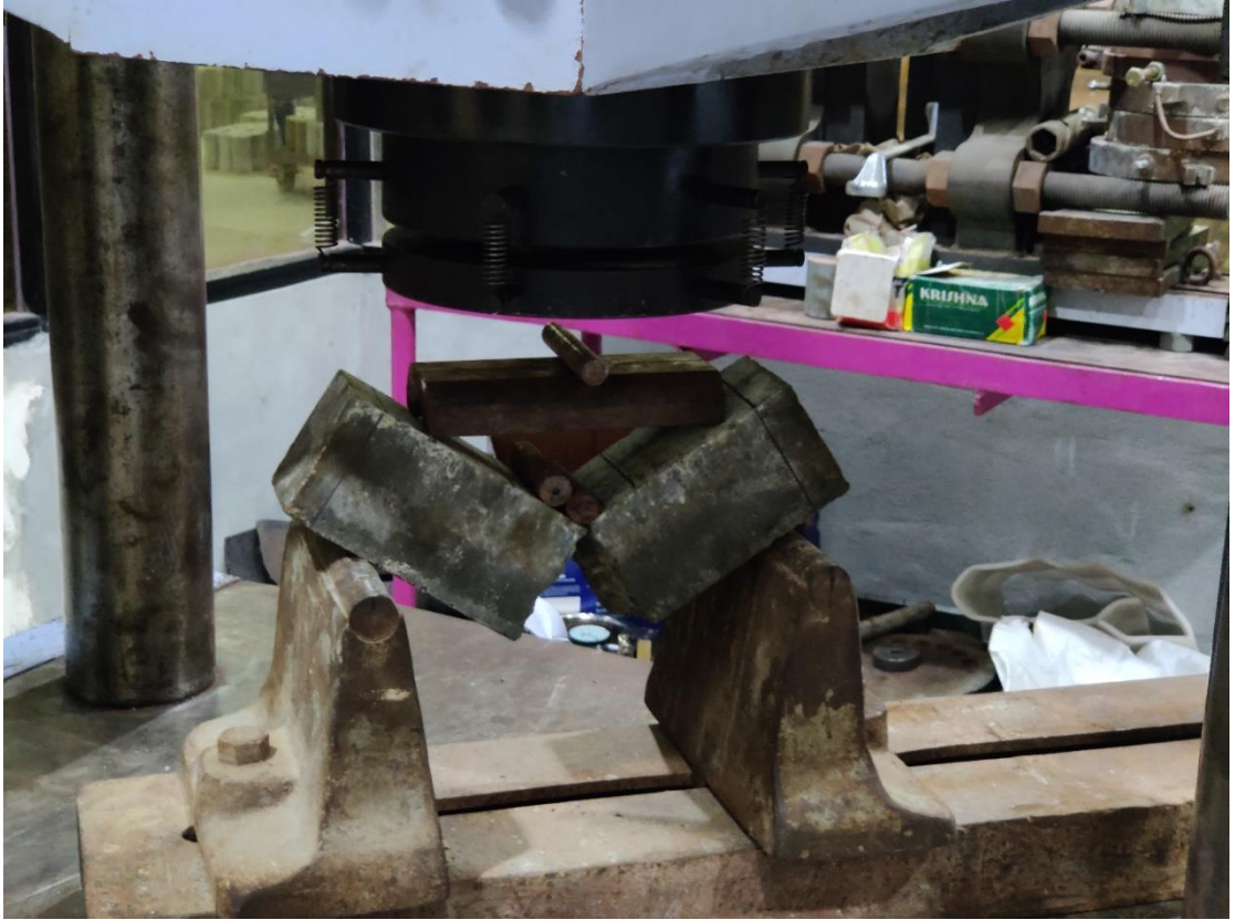
Fig. 4.8: Flexural failure of R100A10F0 concrete mix
