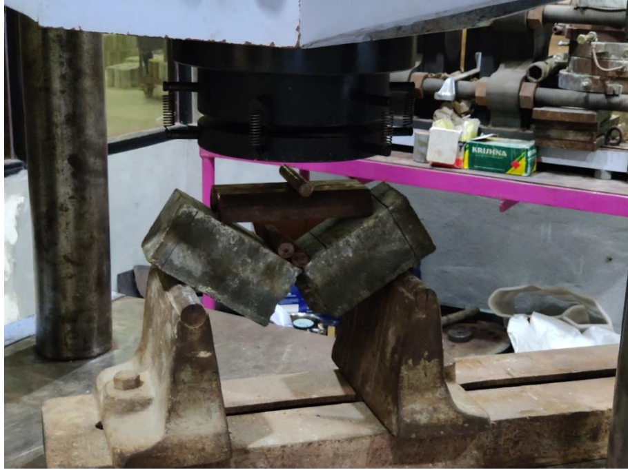
Fig 3.11: Failure by Flexural test (R100A10F0)
