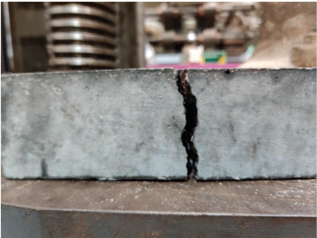
Fig. 4.9: Flexural failure of R100A10F0.2 concrete mix
