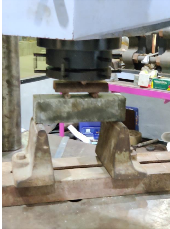
Fig. 3.10: Three Point Loading of Flexural Strength
