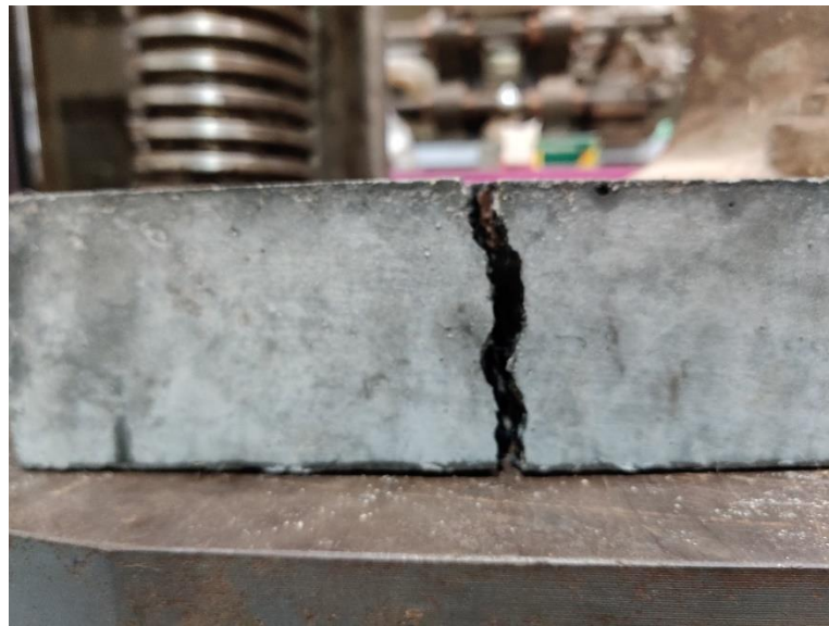
Fig 3.12: Failure by Flexural Test (R100A10F0.35)
