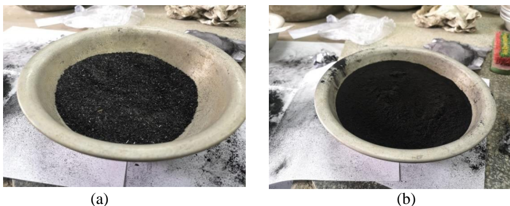
Fig. 3.2: Rice Husk Ash (a) Before Grinding and (b) After Grinding
