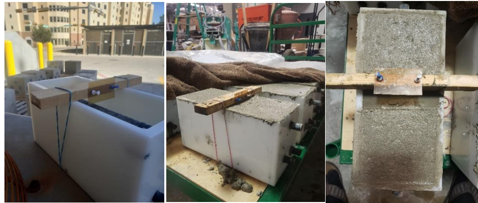
Series 2: Crack introduction
