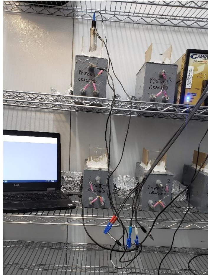
Microcell corrosion measurement
