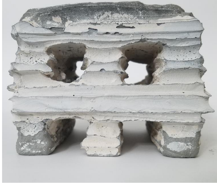
Openings at multiple layers
