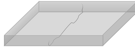
Bottom-Top Transverse crack
