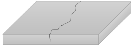
Top-Bottom Transverse crack
