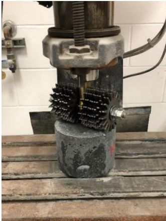
Abrasion resistance testing (left) and samples after abrasion (right)
