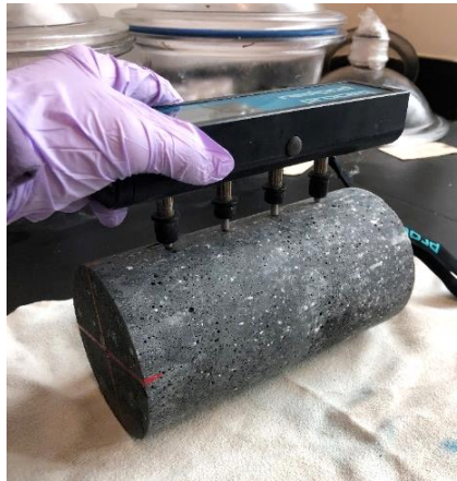
Surface resistivity testing
