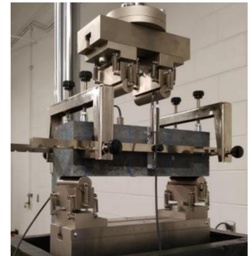
Inferred Tension Bending Test Setup
