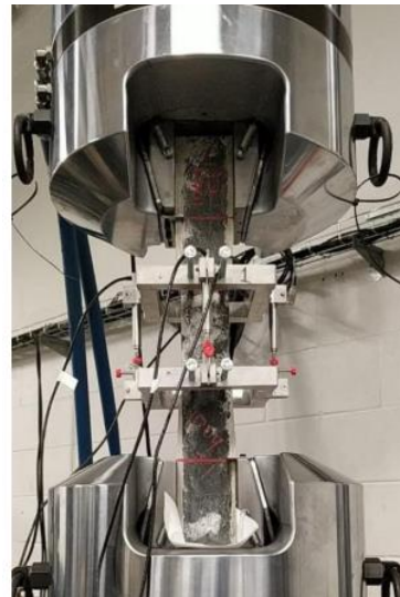
Uniaxial Tensile Strength Test Setup
