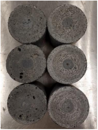
Abrasion resistance testing (left) and samples after abrasion (right)
